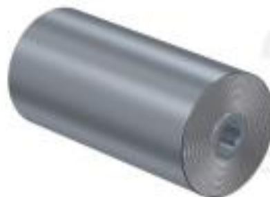
FIGURE 4.4 The metal foil and Mylar sandwich shown in Figure 4.3 can be rolled up with an insulating layer to produce a capacitor with a compact geometry.
