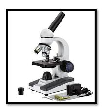
Microscopes magnify things. They make them look bigger than they really are. Many things in science can be studied under a microscope. Light microscopes have been used for a long time. A light microscope uses two glass lenses. The lenses are inside a short tube. A light bulb shines under the object you are looking at. It helps you see the object clearly. Little knobs like wheels can be turned to make the view sharp and clear.
