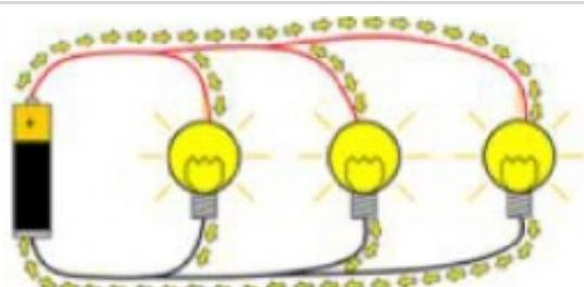
A  Series circuitB  Parallel circuit
