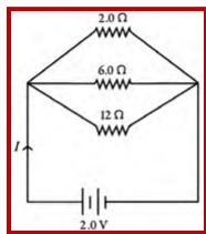
For the circuit shown in the figure, I = 0.50 A and  $R = 12 \Omega$ . What is the value of the emf  $\varepsilon$ ?
