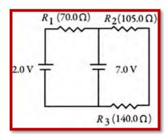
For the circuit shown in the figure, what is the current through resistor R3?
