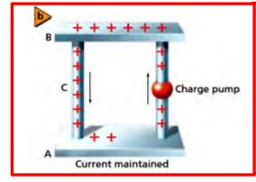
Agenerator pumps the positive charges back to the positive plate and maintains the current
