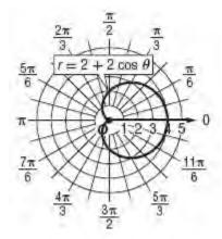
**b.** No; sample answer: The given point is on the negative *x*-axis, directly behind the microphone. The polar pattern indicates that the microphone does not pick up any sound from this direction.
