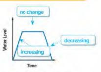
water is turned off and the water level does not change. Finally, the drain plug is pulled and the water level decreases at a constant rate until the water level is zero.
