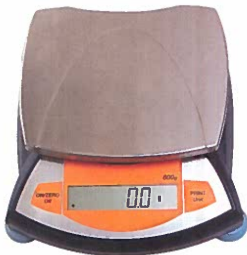
Figure 12 Accuracy is checked by zeroing an instrument before measuring.
