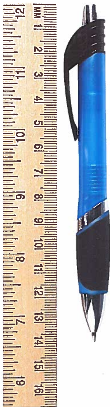
Figure 8 The student measuring this pen recorded the length as 138.1 mm.
