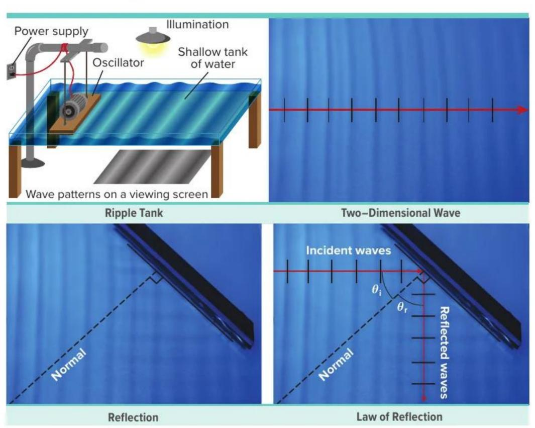
Figure 18 The ripple tank produces uniform waves that are useful for modeling wave behavior.
