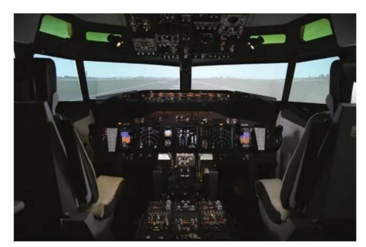
Figure 5 This is a flight simulator used to help train pilots. The image mimics what the pilot would see if flying a real plane.
