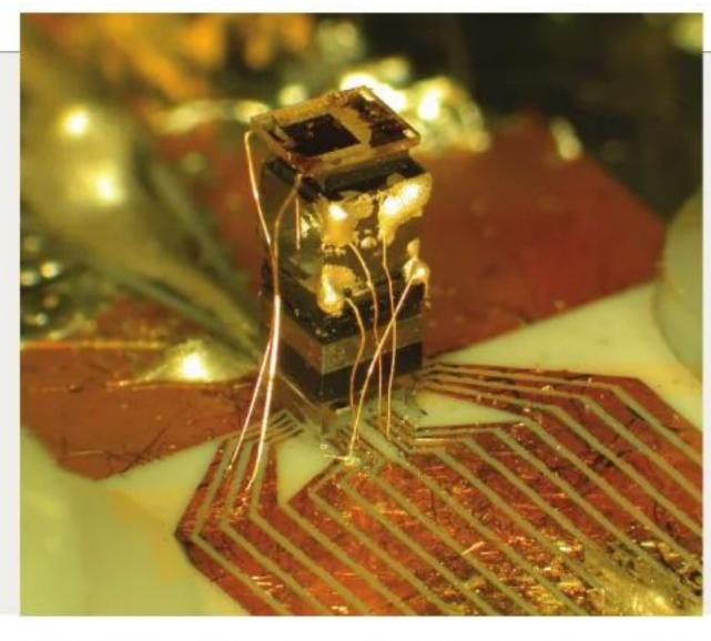
Chip-scale atomic clocks (CSACs) allow for astoundingly accurate and precise time-keeping in a very small package.
