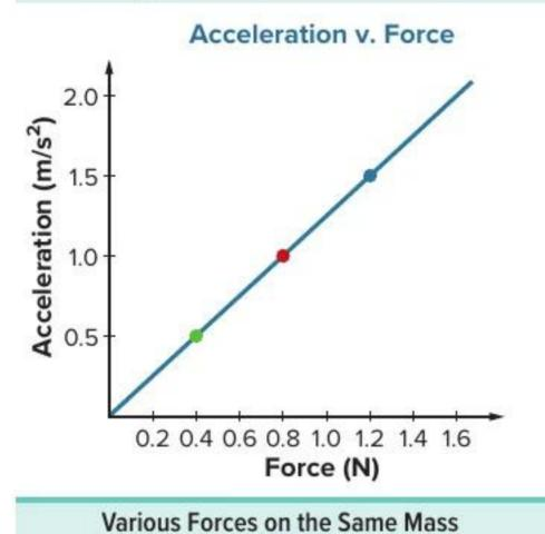
Figure 5 A spring scale exerts a constant unbalanced force on the cart. Repeating the investigation with different forces produces
