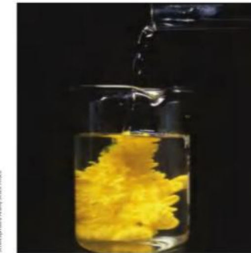
Figure 17 When clear solutions of lead(II) nitrate and potassium iodide mix, a reaction takes place and a yellow solid, lead(II) iodide, appears. The yellow solid that is produced in the chemical reaction is called a precipitate.
