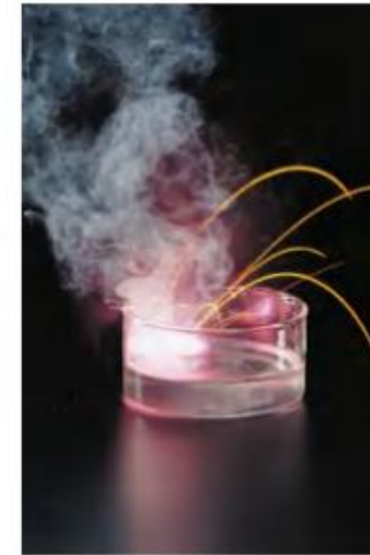
Figure 4 Alkali metals are very reactive. For example, the vigorous reaction between potassium and water releases enough thermal energy to ignite the hydrogen gas that forms.
