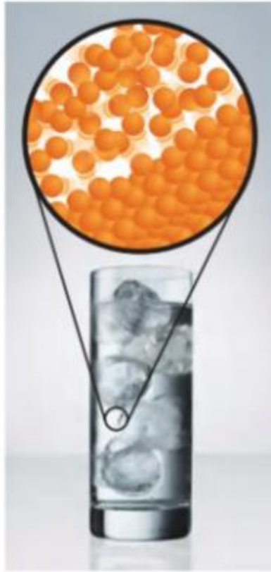
Figure 4 When ice is placed in water, energy from the particles of the liquid water is transferred to the particles of solid ice, melting the ice and cooling the water.
