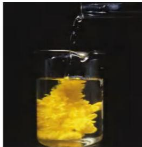
Figure 17 When clear solutions of lead(II) nitrate and potassium iodide mix, a reaction takes place and a yellow solid, lead(II) iodide, appears. The yellow solid that is produced in the chemical reaction is called a precipitate.
