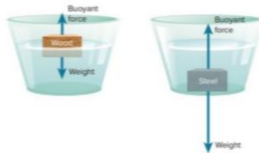
Figure 13 The steel block sinks because the buoyant force from the fluid is less than the gravitational force on the object. When the buoyant force is the same as or greater than the gravitational force—as with the wooden block—the object floats.
