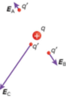
Figure 16 An electric field surrounds particle q . The forces exerted on a positively charged test particle ( q' ) at locations A, B, and C are represented by force vectors. The vectors represent the magnitude and direction of the force from the electric field on the test particle at that point.
