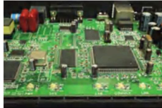
Figure 29 A computer circuit board uses many capacitors in its operation. The gray cylinders, the disk-shaped objects, and the tiny colored tear-drop shaped objects are all capacitors.
