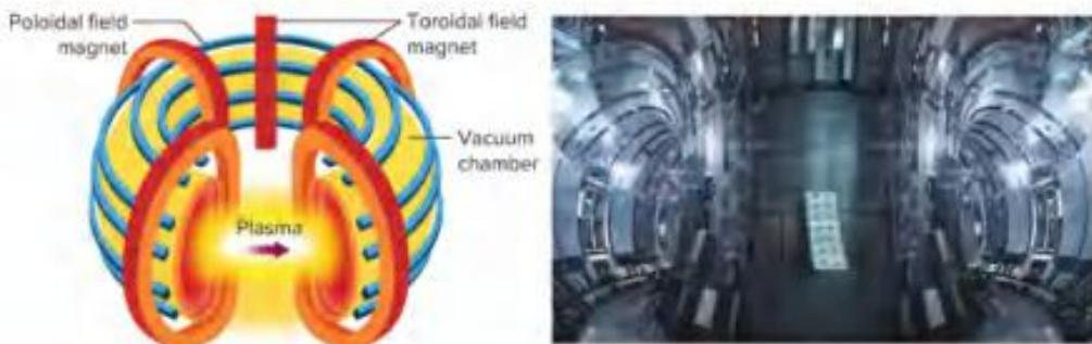
**Figure 23** A tokamak reactor, a ring-shaped reactor, uses strong magnetic fields to contain the intensely hot fusion reaction and keep it from direct contact with the reactor interior walls. The poloidal magnets follow the shape of the reactor, and the toroidal magnets wrap around the reactor.
