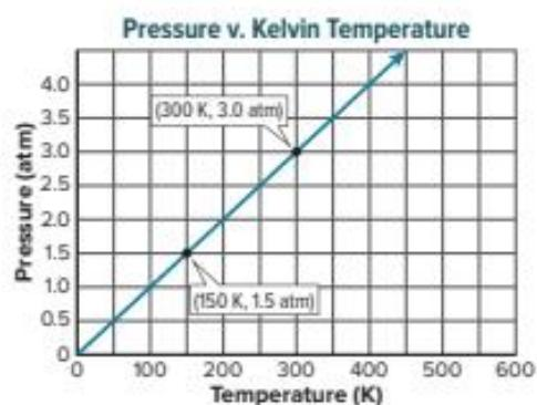
**Figure 3** When the cylinder is heated, the kinetic energy of the particles increases, increasing both the frequency and energy of the collisions with the container wall. The volume of the cylinder is fixed, so the pressure exerted by the gas increases.
