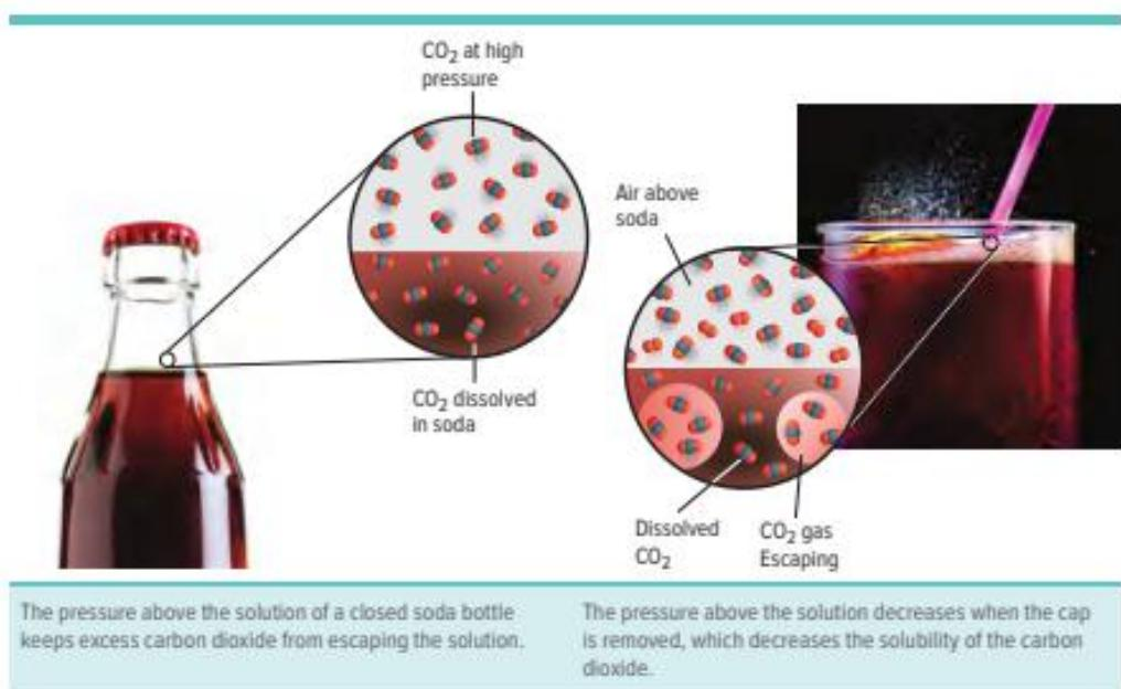
**Figure 19** Carbon dioxide (CO<sub>2</sub>) is dissolved in soda. Some CO<sub>2</sub> also is found in the gas above the liquid.
