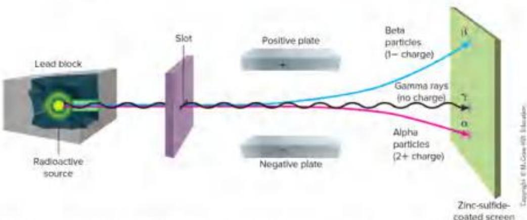
**Figure 2** The effect of an electric field depends on the charge and mass of the radiation. Positively charged alpha particles deflect toward the negative plate. Negatively charged beta particles deflect toward the positive plate. The lighter beta particles undergo the larger deflection. Gamma rays have no charge and are not affected by an electric field.
