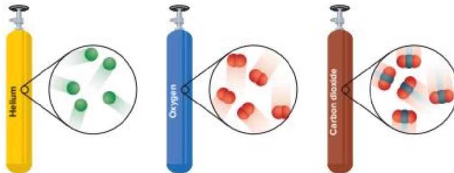
Figure 5 Gas tanks of equal volume that are at the same pressure and temperature contain equal numbers of gas particles, regardless of which gas they contain.
