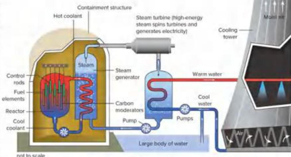
Figure 20 A nuclear reactor produces heat that drives the formation of steam. The energy from the steam spins a turbine, which produces electricity. The steam is eventually cooled and recycled. The water used to cool the steam enters the cooling tower, where steam is released to the atmosphere.
