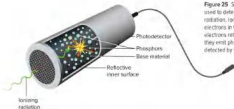
**Figure 25** Scintillation counters are used to detect the presence of ionizing radiation. Ionizing radiation excites the electrons in the phosphors. As the electrons return to their ground states, they emit photons, which are then detected by the photodetector.
