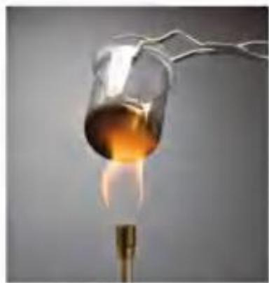
Figure 7 With insufficient oxygen, a Bunsen burner burns with a yellow, sooty flame.
