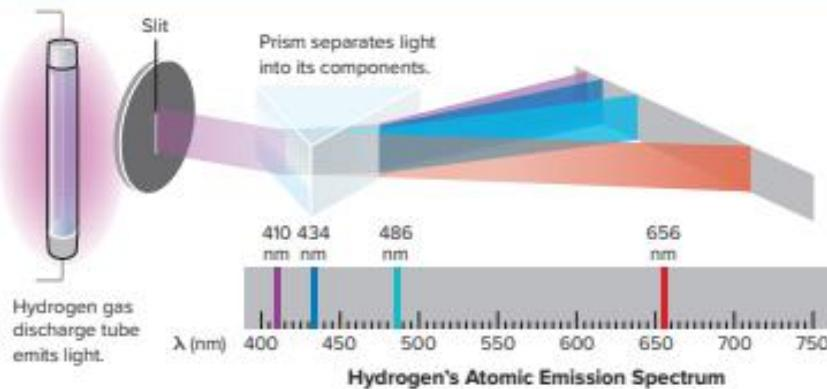
Figure 8 The purple light emitted by hydrogen can be separated into its different components using a prism. Hydrogen has an atomic emission spectrum that comprises four lines of different wavelengths.
