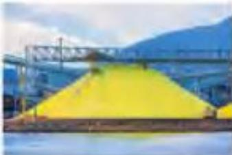
**Figure 9** Sulfur, such as these piles at Vancouver Harbor, can be extracted from petroleum products by a chemical process. Sulfur is also mined by forcing hot water into underground deposits and pumping the liquid sulfur to the surface.
