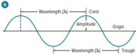
**Figure 2** a. The concentric waves in the water show the characteristic properties of all waves. b. Amplitude, wavelength, and frequency are the main characteristics of waves.
