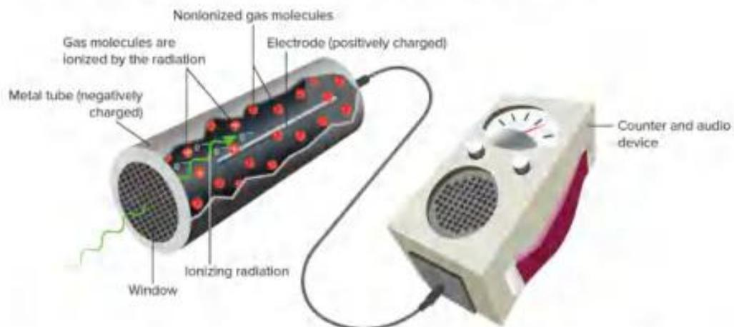
Figure 24 A Geiger counter is used to detect and measure radiation levels. Ionizing radiation produces an electric current in the counter. The current is displayed on a scaled meter, and a speaker produces audible sounds that vary according to the current flow caused by the ionizing radiation.
