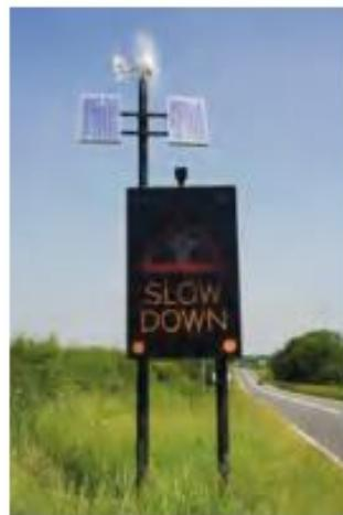
SOLAR ENERGY is sometimes used to power road signs. Photovoltaic cells use the photoelectric effect to convert the energy of light into electric energy.
