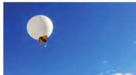
**Figure 4** Weather balloons carry instruments that send data, such as air temperature, pressure, and humidity, to receivers on the ground. As the balloon rises, its volume responds to changes in temperature and pressure, expanding until the sides burst. A small parachute returns the instruments to Earth.
