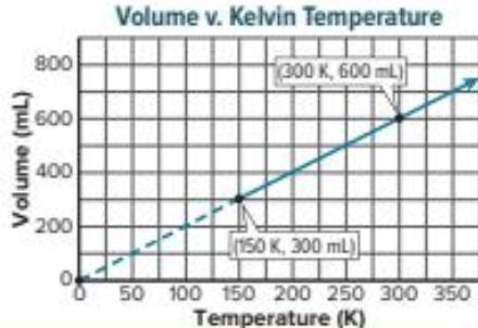
**Figure 2** When the cylinder is heated, the kinetic energy of the gas particles increases, causing them to push the piston outward. The graphs show the relationship of volume to Celsius and Kelvin temperatures.
