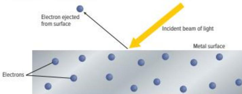
**Figure 7** The photoelectric effect occurs when light of a certain frequency strikes a metal surface and ejects electrons. When the intensity of the light increases, the number of electrons ejected increases. When the frequency (energy) of the light increases, the energy of the ejected electrons increases.
