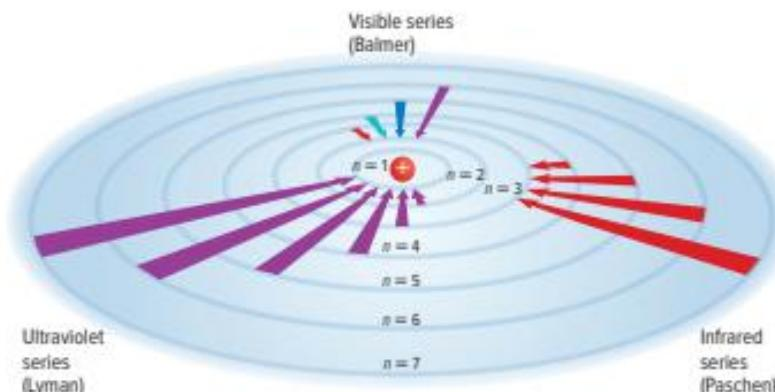
**Figure 11** When an electron drops from a higher-energy orbit to a lower-energy orbit, a photon is emitted. The ultraviolet (Lyman), visible (Balmer), and infrared (Paschen) series correspond to electrons dropping to  $n = 1$ ,  $n = 2$ , and  $n = 3$ , respectively.
