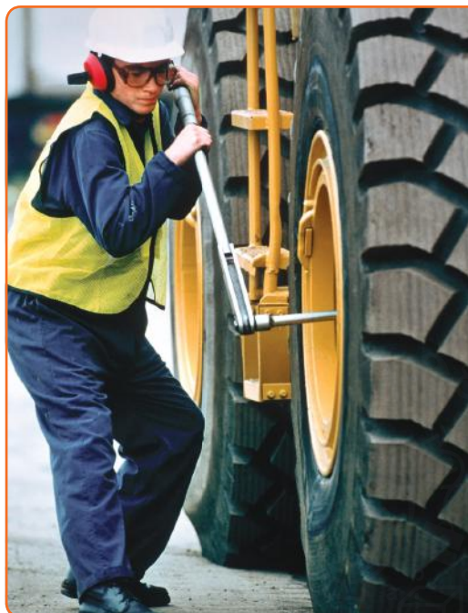
Figure 8 This worker uses a long wrench because it requires him to exert less force to tighten and loosen the nut. The wrench has a long lever arm, and less force is required if the force is applied farther from the axis of rotation (the center of the nut).
