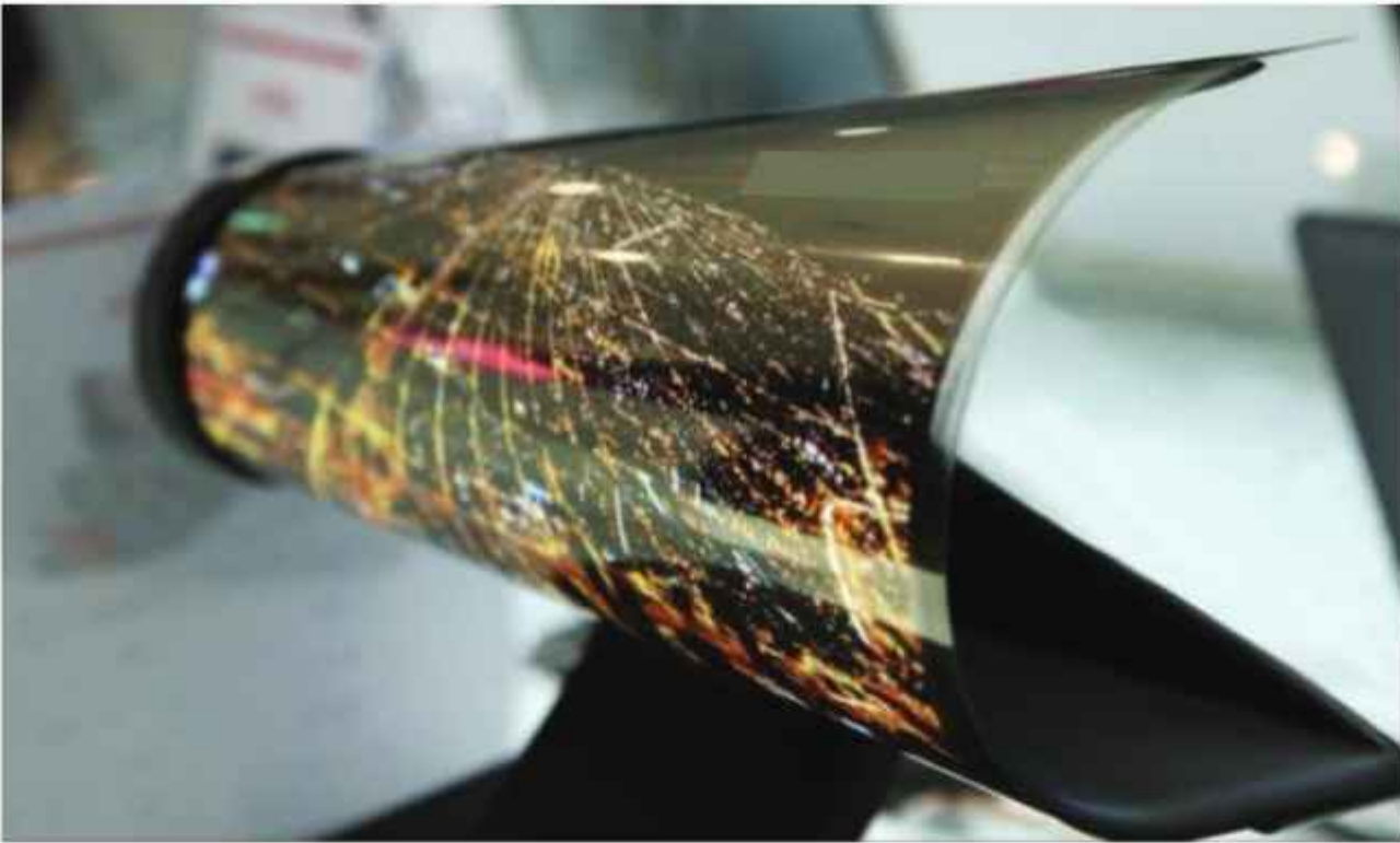
الشكل (11): شاشة (ORGANIC LIGHT EMITTING DIODE: OLED).
