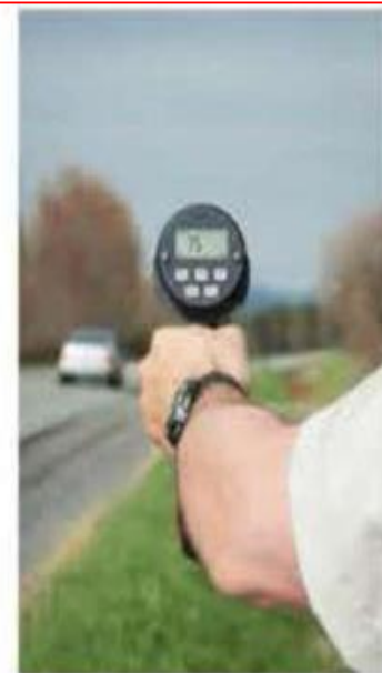
Figure 11 Police use radar guns to measure the speeds of motorists on highways. Radar guns function based on the Doppler effect.
