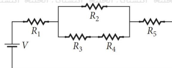
a. What is the equivalent resistance for the circuit?
