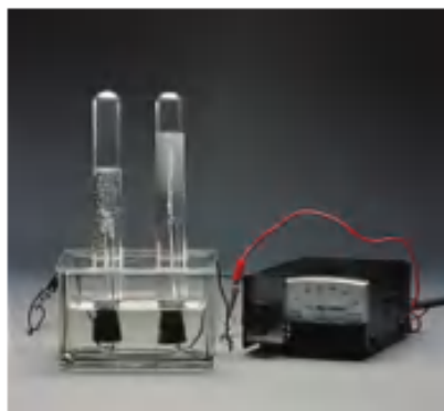
Figure 7 Electrolysis of water produces hydrogen gas that can be used for hydrogen fuel cells.
