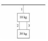
Two masses, 10 kilograms and 30 kilograms, are suspended by massless ropes from the ceiling, as shown in the diagram above. Determine the tension in rope 3.
