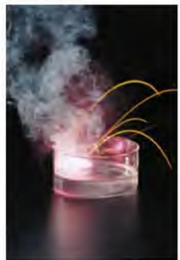
Figure 4 Alkali metals are very reactive. For example, the vigorous reaction between potassium and water releases enough thermal energy to ignite the hydrogen gas that forms.
