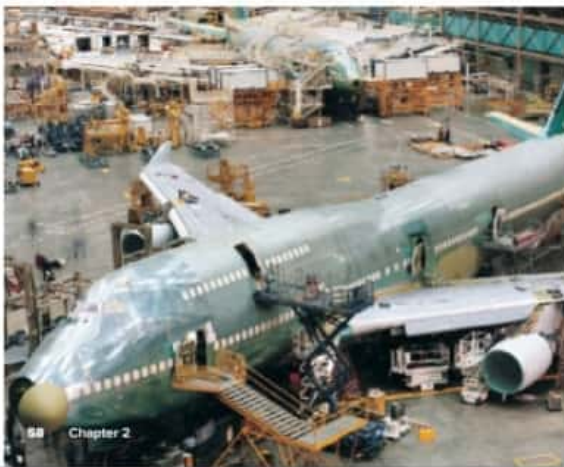
Figure 18: A product, such as this jumbo jet, is manufactured in quantity only after its entire design process is completed.
