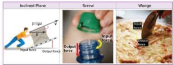
Figure 17 Simple machines do work using one movement. They can change the direction of a force or the amount of force required to perform a task.
