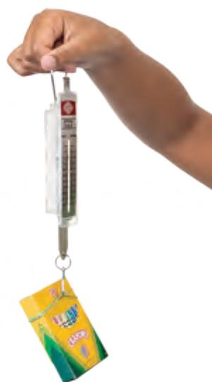
▲ Spring scales are often used in science to determine the weight of an object.
