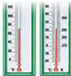
Figure 4 Thermometers measure temperature. Common temperature scales are Celsius, Kelvin, and Fahrenheit.
