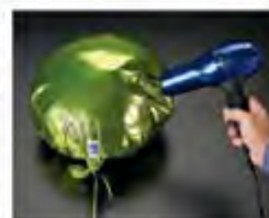
Figure 9 Air inside the balloon increases in volume when the temperature increases.
