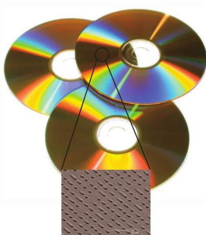
**Figure 16** A CD is a reflection grating, producing a light spectrum. A magnified view of the surface of a CD shows the arrangement of pits and lands.
