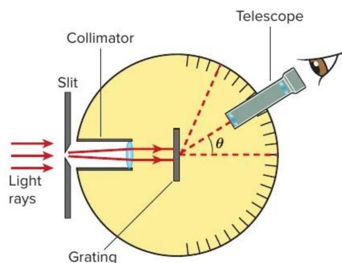
**Figure 17** A grating spectroscopy is used to accurately measure the wavelength of light.
