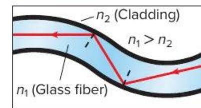
**TOTAL INTERNAL REFLECTION** is used in communication via optical fibers. The light traveling through the transparent fiber always hits the internal boundary of the optical fiber at an angle greater than the critical angle. All the light is reflected, and none of the light is transmitted through the boundary. Light pulses in fiber optic cables carry larger amounts of information over longer distances than other forms of communication. The outer material of each fiber is called cladding.
