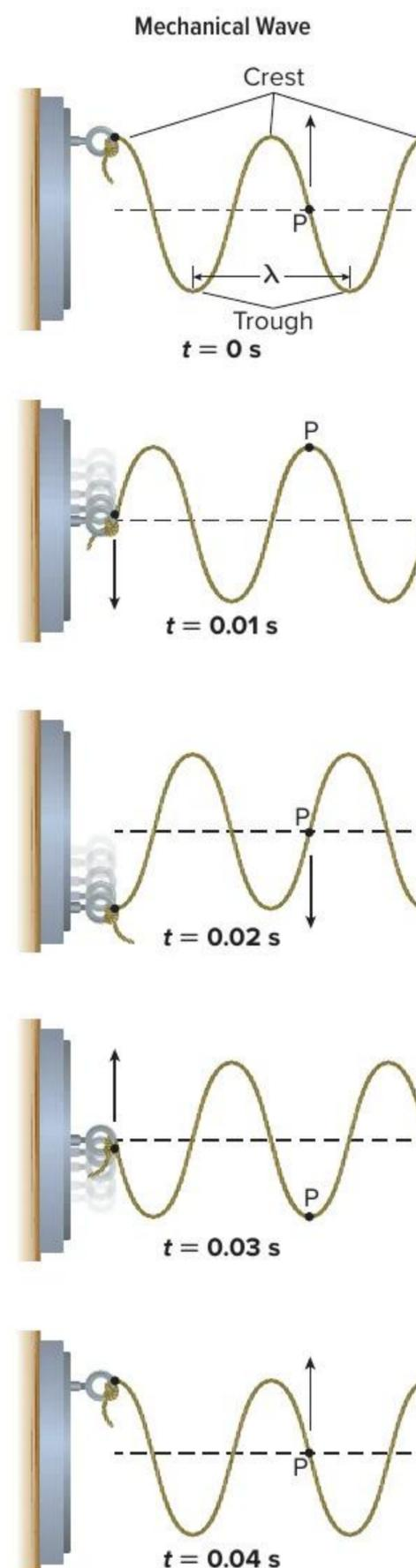
**Figure 9** A mechanical oscillator moves the left end of the rope up and down, completing the cycle in 0.04 s.
