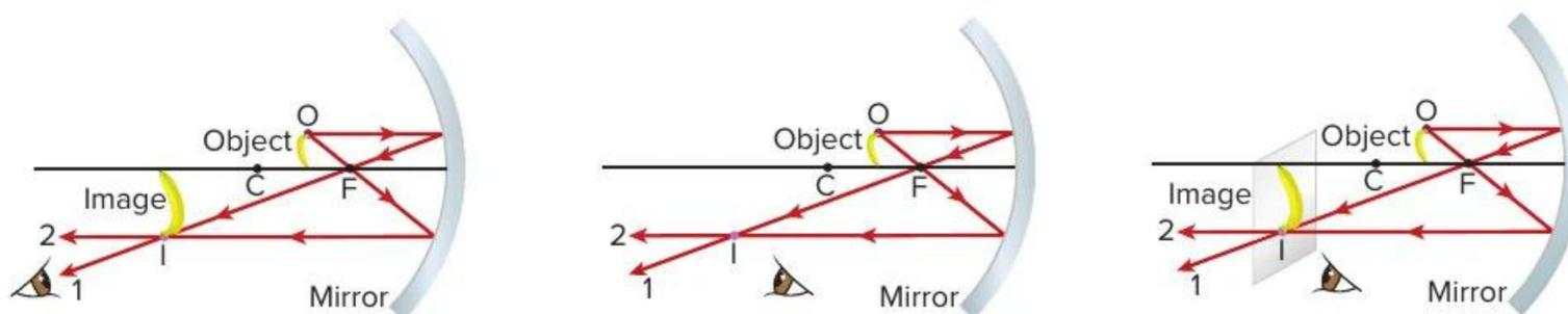
The eye is positioned so that the rays that form the real image strike the eye, allowing the image to be seen.
