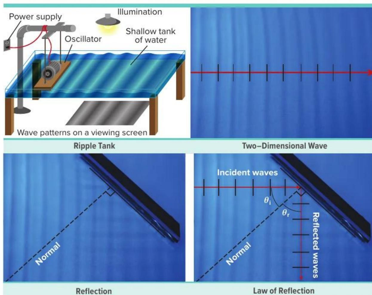
**Figure 18** The ripple tank produces uniform waves that are useful for modeling wave behavior.
