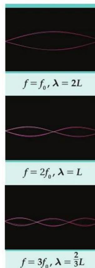
**Figure 16** Interference produces standing waves only at certain frequencies.
