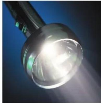
A lightbulb is placed at the focal point of a concave mirror. The parallel reflected rays are evident in this flashlight beam.
